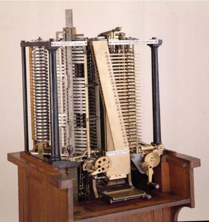
section of the "mill" of the Analytical Engine (above) and Difference engine (below). Reconstructed by his son Henry
