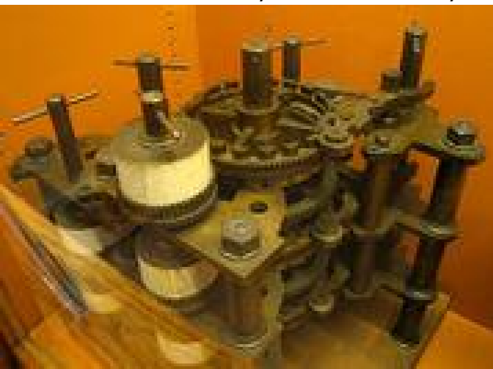
section of the "mill" of the Analytical Engine (above) and Difference engine (below). Reconstructed by his son Henry
