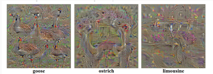
Figure: Input optimization saliency maps of a deep CNN trained on imagenet as shown in [SVZ13].
